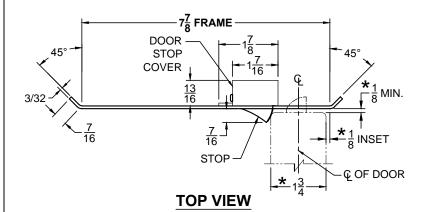
STOP IS SPRING LOADED MAKING PART NON-HANDED BUT INSTALLATION IS STILL HANDED
