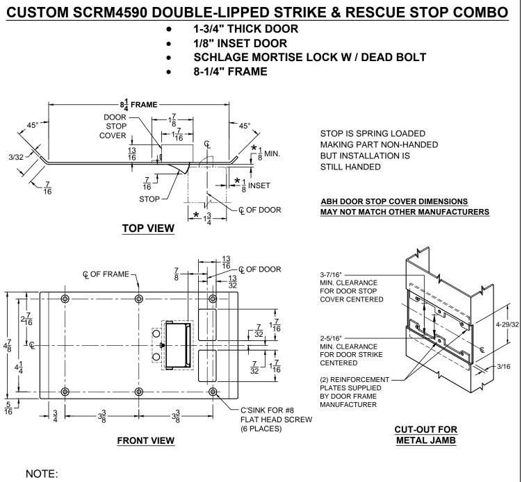
1. HORIZONTAL CENTERLINE OF PLATE TO MATCH HORIZONTAL CENTERLINE OF CUTOUT.
