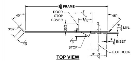
STOP IS SPRING LOADED MAKING PART NON-HANDED BUT INSTALLATION IS STILL HANDED
