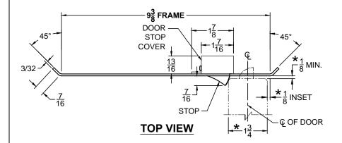
STOP IS SPRING LOADED MAKING PART NON-HANDED BUT INSTALLATION IS STILL HANDED
