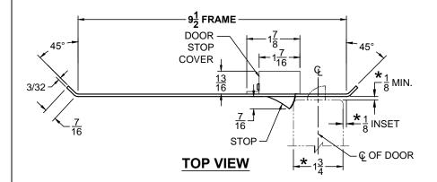
STOP IS SPRING LOADED MAKING PART NON-HANDED BUT INSTALLATION IS STILL HANDED
