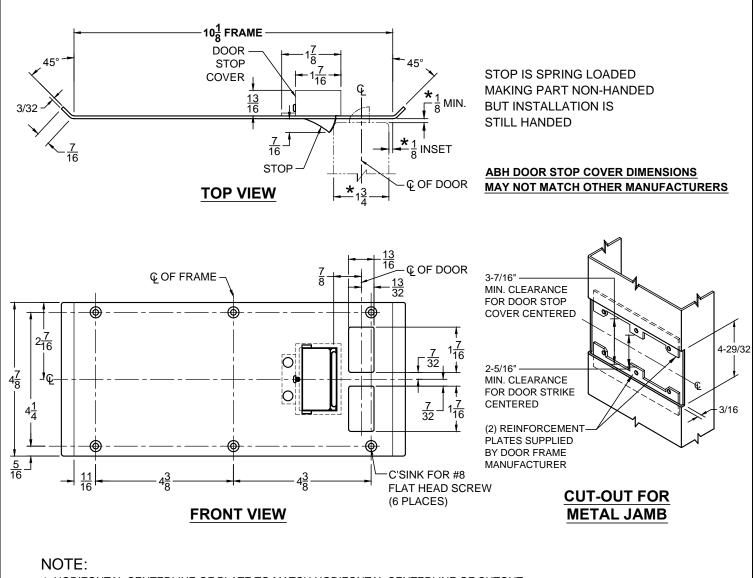
1. HORIZONTAL CENTERLINE OF PLATE TO MATCH HORIZONTAL CENTERLINE OF CUTOUT.
