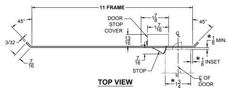
STOP IS SPRING LOADED MAKING PART NON-HANDED BUT INSTALLATION IS STILL HANDED
