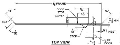
STOP IS SPRING LOADED MAKING PART NON-HANDED MIN. BUT INSTALLATION IS STILL HANDED
