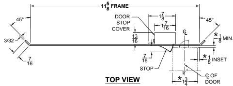
STOP IS SPRING LOADED MAKING PART NON-HANDED MIN-BUT INSTALLATION IS STILL HANDED
