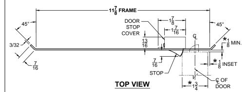
STOP IS SPRING LOADED MAKING PART NON-HANDED BUT INSTALLATION IS STILL HANDED
