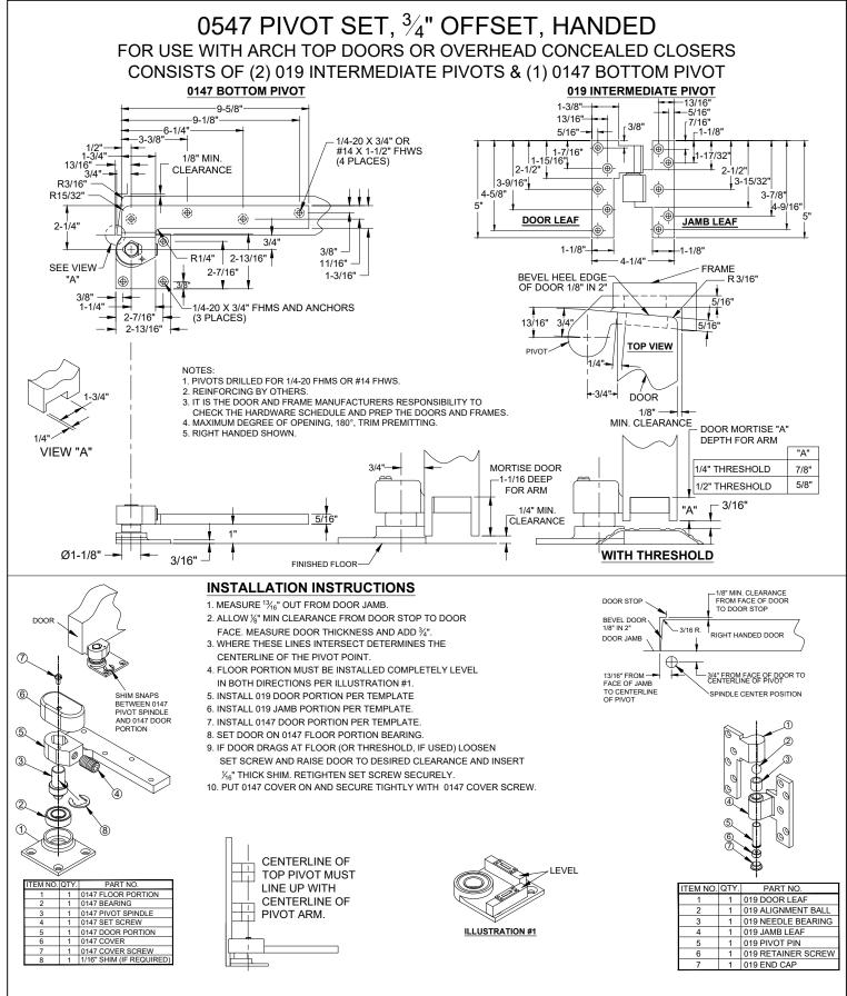
**Disclaimer:** This template is to be used for installation, as shown, of said product and is not suitable for every application method. Custom applications, where door sizes, weights and conflicting hardware are a factor, need to be addressed with ABH and proper instructions provided. ABH is not liable for failure or performance of the product due to improper installation methods and/or use. Improper use and/or installation of this product will void the standard warranty.
