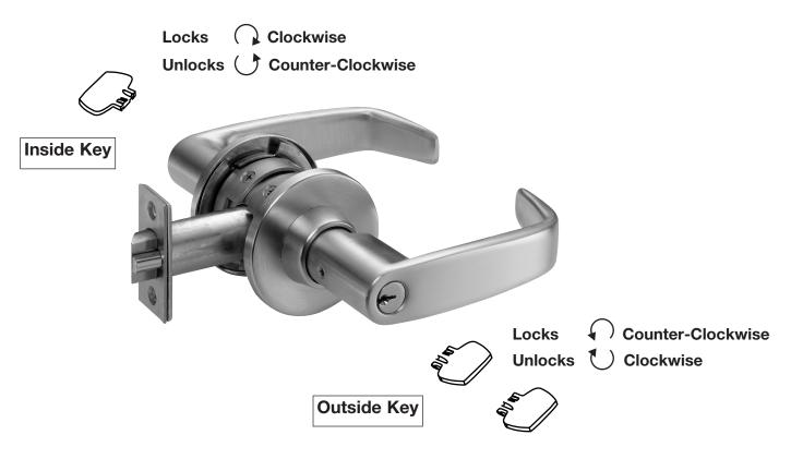
When inside key locks outside lever, outside key only retracts the latchbolt. Outside key must be rotated back completely clockwise before removing the key.
