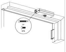
3. Remove dial from Hold Open arm and install separate arms.
