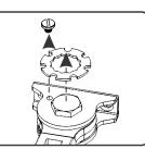
4. Install soffit plate and mount closer.
