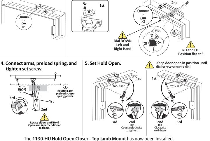
The 1130-HU Hold Open Closer - Top Jamb Mount has now been installed. Go to page 2 for closer adjustments and decorative cap or cover installation.
