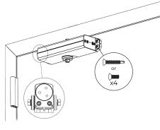
3. Remove dial from Hold Open arm and install separate arms.
