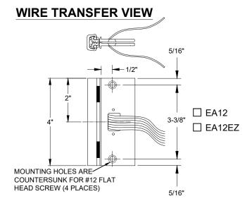
GEAR HINGE 4 INCH REMOVABLE SECTION RIBBON CABLE INSTALLATION-01.DWG
