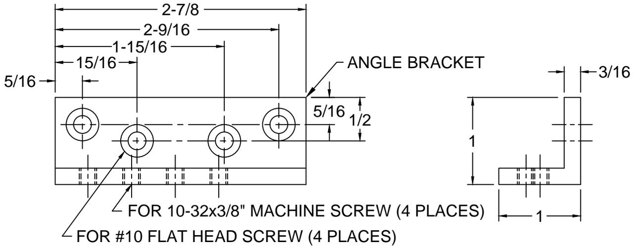
THE ANGLE BRACKET IS SECURED TO THE HEADER WITH WOOD OR MACHINE SCREWS. THE JAMB BRACKET FASTENS TO THE ANGLE BRACKET WITH MACHINE SCREWS. THE CHANNEL MOUNTS ON THE DOOR WITH SEX BOLTS. REVERSE INSTALLATION METHOD IS NOT RECOMMENDED FOR EXTERIOR DOORS OPENING OUT.
