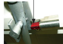
STOP SHOWN BEFORE DOOR IS FULLY OPENED
