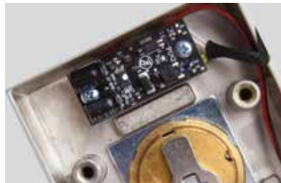
SMARTSENSE control board automatically accepts different input voltages: 12-24VDC, 12-24VAC
