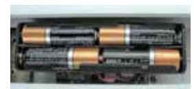
pdqSMART Electronics Package and Battery Pack Securely Located in the Filler End of the Exit Device Touchbar Rail.
