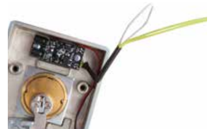
To convert from FAIL SECURE to FAIL SAFE, simply cut the looped white wire
