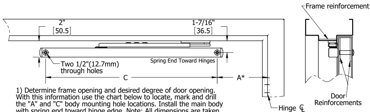
1) Determine frame opening and desired degree of door opening. With this information use the chart below to locate, mark and drill the "A" and "C" body mounting hole locations. Install the main body with spring end toward hinge edge. Note: All dimensions are taken from the hinge center line.
