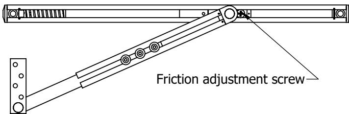
Using a flat head screwdriver, turn the friction adjustment screw clockwise to increase the friction and counter-clockwise to lower the friction.
