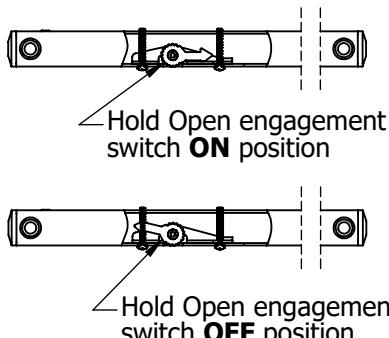
Using a Philips screwdriver, turn the hold open adjustment screw clockwise to increase the hold-open tension and counter-clockwise to lower the tension.
