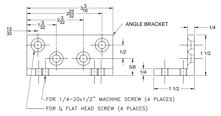
THE ANGLE BRACKET IS SECURED TO THE HEADER WITH WOOD OR MACHINE SCREWS. THE JAMB BRACKET FASTENS TO THE ANGLE BRACKET WITH MACHINE SCREWS. THE DOOR BRACKET MOUNTS ON THE DOOR WITH THROUGH SCREWS AND GROMMET NUTS
