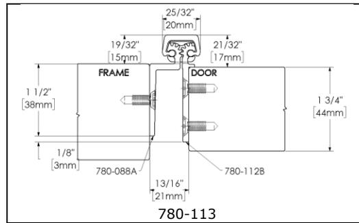
ROTON Models 780-113 is an Aluminum Continuous Geared Concealed Leaf Hinge. Clearance required between the hinge edge of the door and the frame is 13/16" (21mm). "HD" models have additional bearings and fasteners for heavy-duty application.
