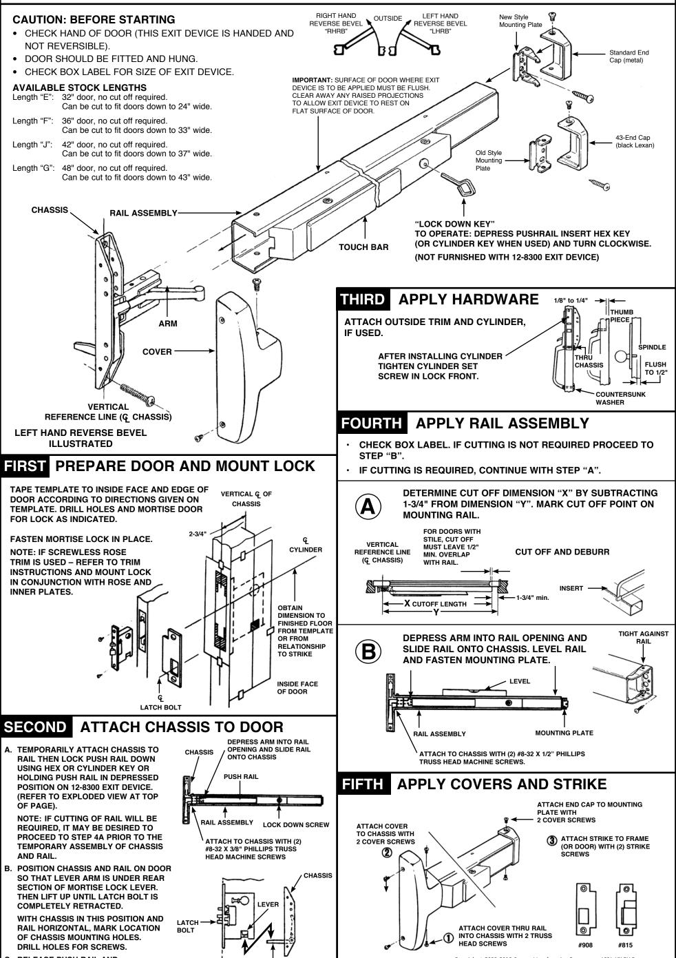
**RELEASE PUSH RAIL AND** C. **DISASSEMBLE CHASSIS FROM RAIL.** THEN MOUNT CHASSIS ON DOOR.
