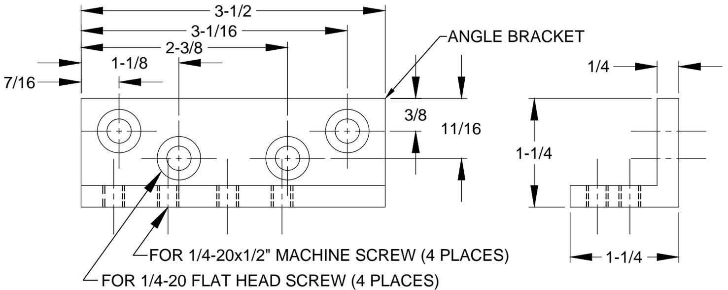
THE ANGLE BRACKET IS SECURED TO THE HEADER WITH WOOD OR MACHINE SCREWS. THE JAMB BRACKET FASTENS TO THE ANGLE BRACKET WITH MACHINE SCREWS. THE CHANNEL MOUNTS ON THE DOOR WITH SEX BOLTS. REVERSE INSTALLATION METHOD IS NOT RECOMMENDED FOR EXTERIOR DOORS OPENING OUT.
