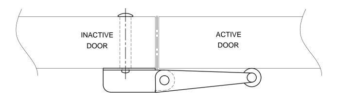
THE CARRY BAR WILL PUSH THE ACTIVE DOOR OPEN ALONG WITH THE INACTIVE DOOR AND ALLOW THE COORDINATOR MECHANISM TO ENGAGE BOTH DOORS AND TO COORDINATE THEM TO CLOSE CORRECTLY.
