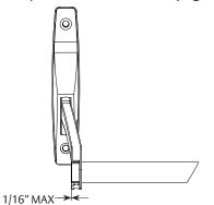
3. Drill 3/16" hole thru one side of bar using hole in arm to locate. (Figure 4)
