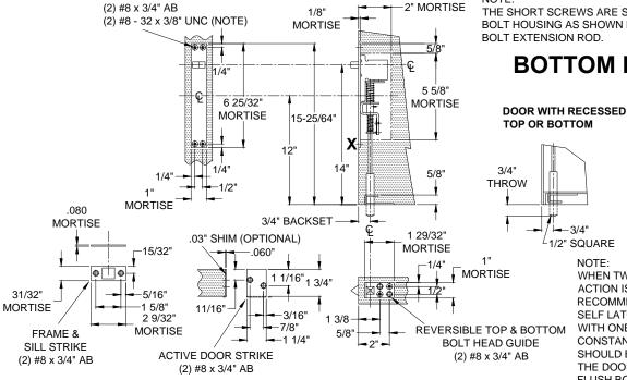
THE SHORT SCREWS ARE SEATED INTO THE HOLES OF THE BOLT HOUSING AS SHOWN MARKED "X", WHERE FACES THE
