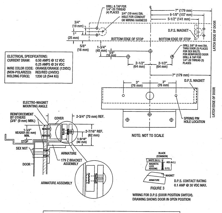
NOTE: REINFORCEMENT AND STRUCTURE IS REQUIRED TO WITHSTAND 1200 LBS, LOAD
