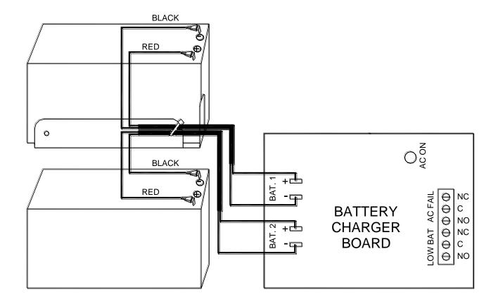
Place one of the two supplied batteries in the lower-left corner of the enclosure. Place the second battery on the shelf above the other battery. Tilt the top of each battery forward to gain access to the terminals. Connect the two pre-assembled 2-conductor cable leads to the battery terminals as shown above.
