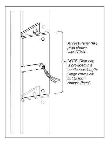
**PREP:** SELECT geared continuous hinges can be prepared with hinge leaf panels to allow easy access to electrical components while preserving gear cap's appearance.
