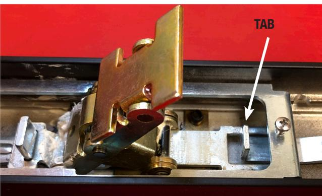
**6.** Once plunger bracket is past tab tighten screw all the way to prevent the bracket from moving forward.
