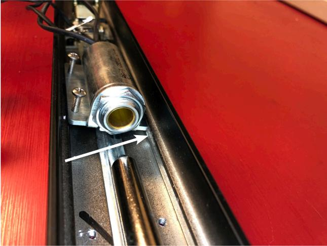
8. Press down on the solenoid mount to pop in the other side of the solenoid mount into the middle groove.
