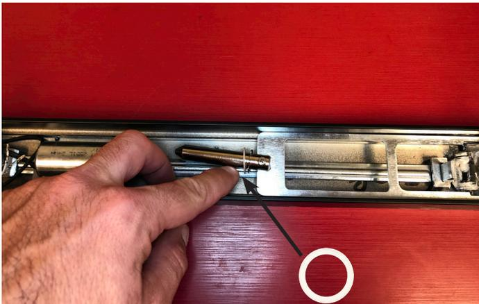
10. Move solenoid mount up towards plunger & install remaining (2) screws to mount. DO NOT TIGHTEN!
