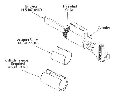
Note: 4700LN and NexTouch® series manufactured since 2021 no longer require the cylinder sleeve. The sleeve is only required on legacy models of these series.
