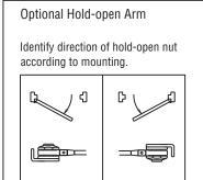
Optional Hold-open Arm Identify direction of hold-open nut according to mounting.
