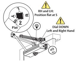
4. Connect arms, preload spring and tighten set screw.
