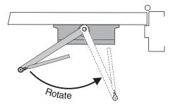
7. Remove arm and attach as shown.
