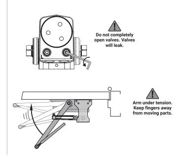
I. Connect arms, preload spring, and tighten set screw.
