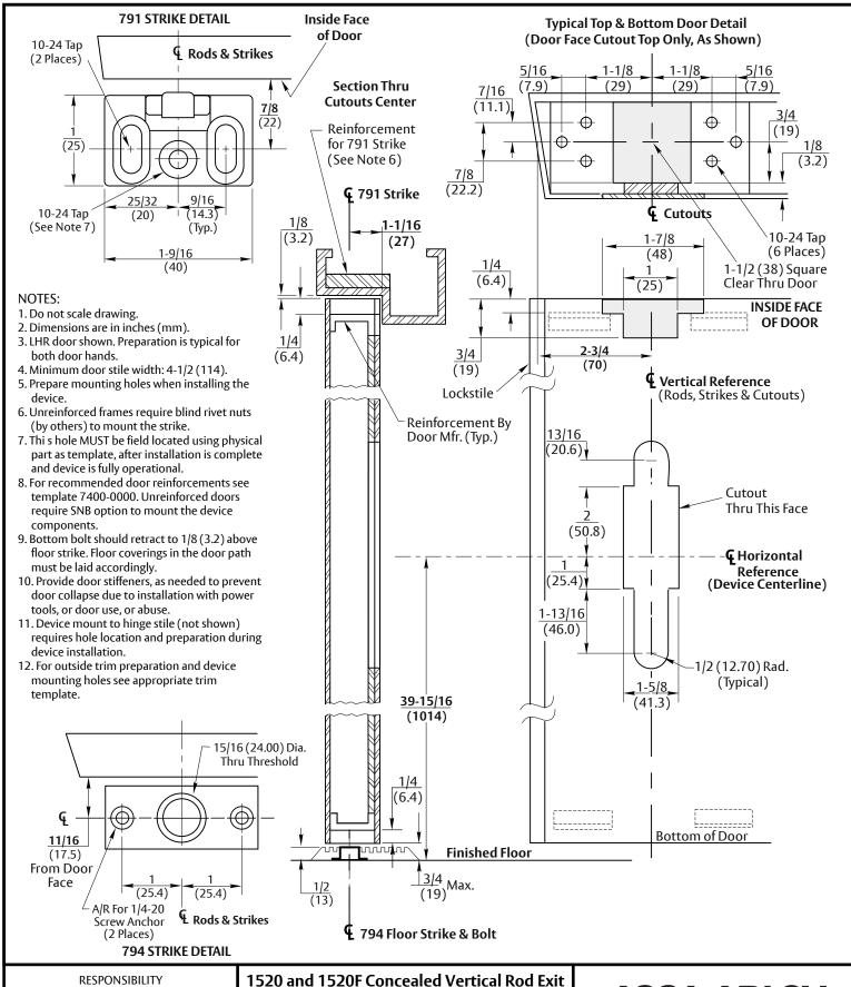
DOOR AND FRAME MANUFACTURERS ARE RESPONSIBLE FOR PROVIDING ADEQUATE CONSTRUCTION OR REINFORCEMENTS FOR PROPER INSTALLATION OF HARDWARE SHOWN. ALL ARCHITECTURAL BUILDERS HARDWARE MUST BE INSTALLED ON PROPERLY REINFORCED DOORS AND FRAMES, REGARDLESS OF TYPE, MATERIAL, OR METHOD OF CONSTRUCTION.
