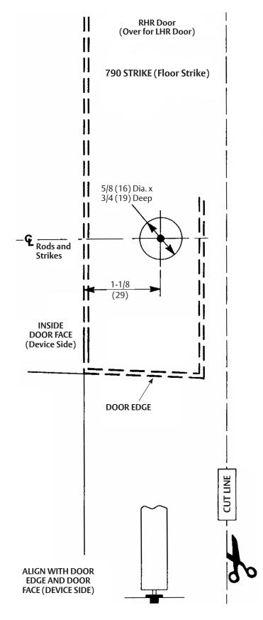
**Caution:** Office copiers, printers and facsimile machines may change the size of a drawing and make the template inaccurate to use as a door marker.
