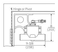
**Corner Mounting, Extra Drop - 2950 Corner Bracket:** For use with a separate overhead door holder. Drops closer 1" (25mm) lower than 1950 Standard Drop Corner Bracket to permit mounting of an overhead holder. Permits door openings to 180°. Minimum soffit width 1-3/8" (35mm).
