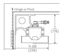
**Corner Mounting, Standard Drop - 1950 Corner Bracket:** For use where door is required to open to 180°. Minimum soffit width 1-3/8" (35mm).
