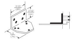
**Flush Transom - 293L Angle Bracket:** For use where flush transom conditions prevent installation of the standard hold open soffit plate. Used for parallel hold open arms.
