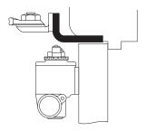
**Molded/Bull Nose Trim - 292 Bracket:** For use where the door frame has molded or bull nose trim which will not accept a standard hold open shoe. It is mortised into the frame rabbet, and projects beyond the face of the frame. It will accommodate a rabbet up to 2" (51mm) deep. This bracket is used in combination with the standard hold open mounting shoe.
