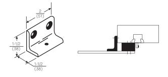
**Narrow Frame - 890 Support Bracket:** For use where the frame is narrow, and the soffit plate cannot be mounted directly to the frame soffit or rabbet. Used in combination with the 891 Spacer Block on blade stop frames to provide extra support and needed clearance of the blade stop.
