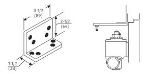
**Flush Transom - 589L Angle Bracket:** For use where rabbeted or flush transom conditions prevent installation of a soffit plate. Used in combination with the 289 soffit plate, or it may be used in combination with the 290 soffit plate when it is necessary for the closer arm to clear a separate overhead door holder.
