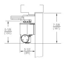
Body mounting holes are spaced 4-1/8" (105mm) horizontally and 1-3/8" (76mm) vertically.
