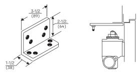
**Flush Transom - 589L Angle Bracket:** For use where rabbeted or flush transom conditions prevent installation of a soffit plate. Used in combination with the 289 soffit plate, or it may be used in combination with the 290 soffit plate when it is necessary for the closer arm to clear a separate overhead door holder.
