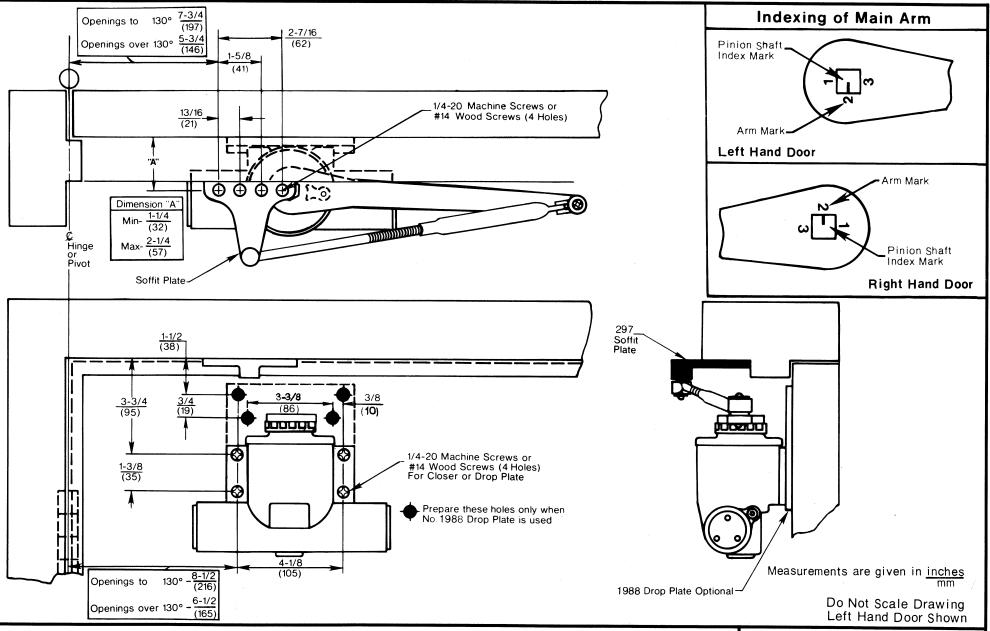
PA1900 Series Door Closers with 297 Soffit Bracket Parallel Arm Non Hold Open Installation With or without No. 1988 Drop Plate Closer Sizes PA1902/4 or PA1905/6
