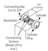
Connecting bar and screws available for 2-1/4" to 3-1/4" (57mm to 82mm) doors.
