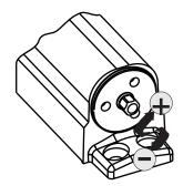
(Use 5/16" Socket or Adjustable Wrench for this Adjustment)
