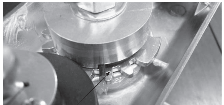
Spring orientation for right hand reverse operation
