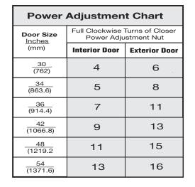
**NOTE**: Maximum of 15 turns (360°) of Power Adjustment Nut. Closer is shipped set at lowest power setting.
