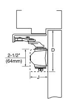
Mounting holes are spaced: 3/4" (19mm) vertically x 8" (203mm) horizontally.
