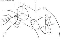
A. Drill 2-1/8" (54mm) hole thru the door. Cut Notches as shown on the template.
