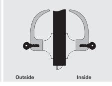
\*Lever handles are Free Wheeling in locked position. Shaded area denotes Free Wheeling lever.
