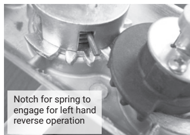
Spring orientation for right hand reverse operation
