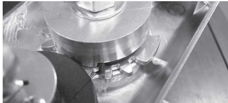
Spring orientation for right hand reverse operation
