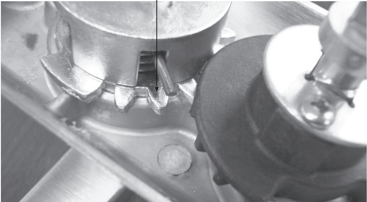
Notch for spring to engage for left hand reverse operation
