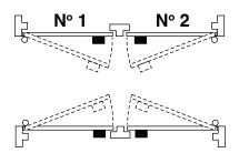
For Doors Opening Outward Use #8 Reverse Bevel Strike (Available Upon Request) Connecting bar and screws available for 2-1/4" to 3-1/4" (57mm to 82mm) doors.
