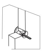
D. Use the button on front of lock case to hold latch in retracted position. Install lock case over the mounting plate making sure the flat connecting bar goes in the slot on the lock case. B. Hold mounting plate against inside of the door. If necessary, shorten the flat connecting bar so it projects 15/32" (12mm) beyond surface of mounting plate.
