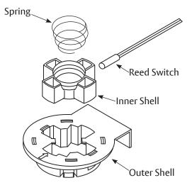
4. Turn Inner Shell on side. Align the inner shell with the diagonal slot in the Outer Shell. Slide the Inner Shell through the Outer Shell.
