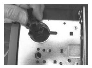
7. Assemble Inner Shell into Outer Shell. Guide the sensor wire out the top of the lock.
