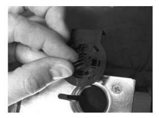
Remove Inner Shell from Outer Shell by gently 3. pressing the Inner Shell upwards from the bottom. Use caution not to damage sensor wires.
