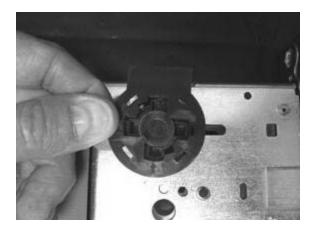
9. Gently press Cylinder Monitoring Assembly into cylinder hole on the new side of the lockbody.
