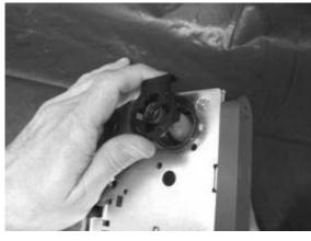
Remove spring from assembly. Use caution not 2. to stretch or otherwise deform the spring.
